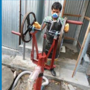
Mechanized gulper Capacity: 60 liters/minute
