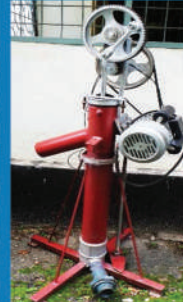
Motorized gulper Capacity: 90 liters/minute
