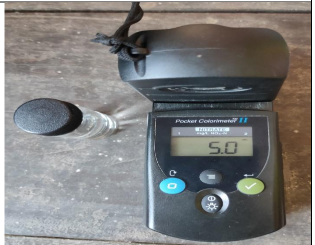
Water Quality Testing using Pocket Colorimeter (for Nitrate)
