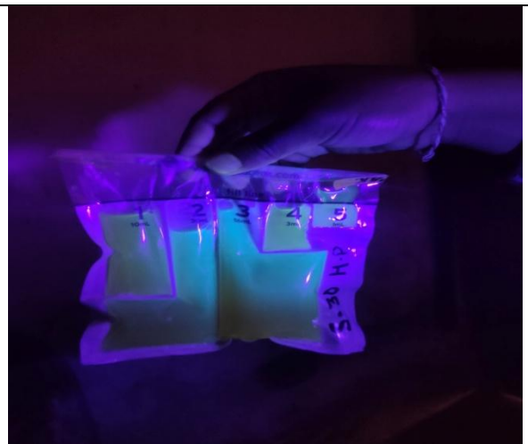
Water Quality Testing using MPN Test Kit
